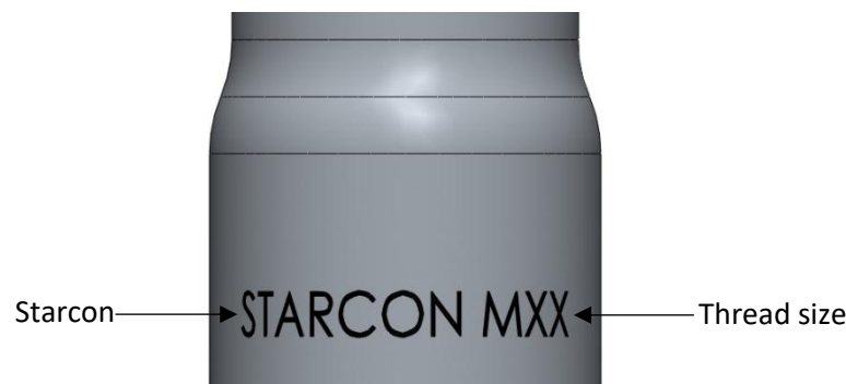
Figure 2 Marking on the cylinder of the Insert for fastening.
