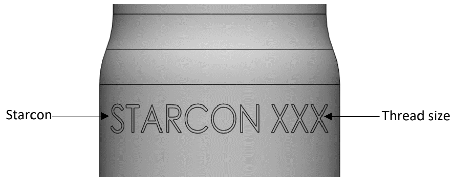
Figure 2 Marking on the cylinder of the Insert for fastening.
