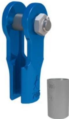
Forged clevis fittings with bolt, nut and cutterpin for fast connection of steel wire rope. Connector shall be used with non-rotating or cat 1. rotation resistant wire rope only.
