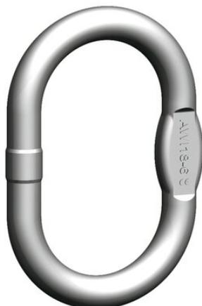
Stamped and suitable for both I- and II-leg assemblies and wire rope slings (similar to DIN 3088- 1989). Its dimensions are similar to DIN 5688-1 and it is tested at 100 % of its load capacity.
