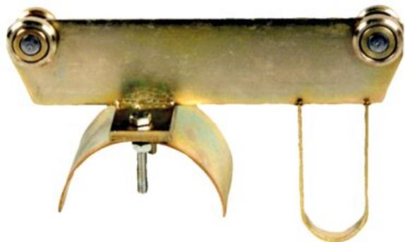
This trolley is pulled along by means of a towing arm fitted to the travelling device and inserted into the stirrup section of the trolley. It cannot be used on curved tracks.
