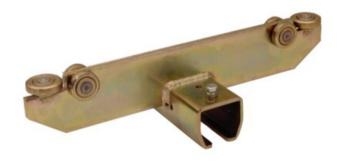
This range of trolleys are fitted with horizontal guide rollers and are used for connecting the moving cross members to the inner side tracks. For standard crane applications it is recommended that only one side of the cross member is fixed allowing the other side to move freely to facilitate track misalignment.
