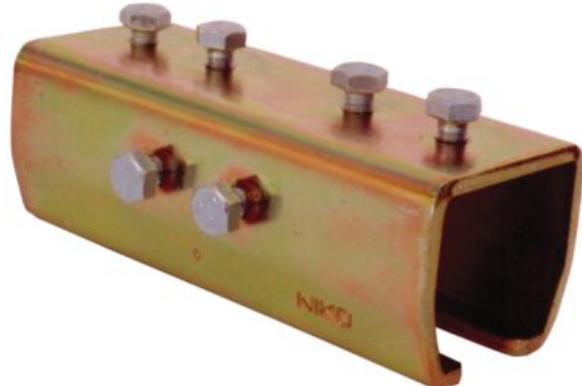
The track sections are joined using the track joint by tightening the top screws first then aligning the profiles by means of the side screws.
