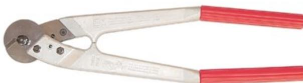
Cut both hard-drawn wire like steel-, copper- and aluminum wires, electric cables and multi wire ropes. The cutting edges are shaped to form a grip of the rope, in shape of a triangle when cutting which prevents un-twisting of the rope end. The edges are made in alloy steel of coromanttype. The cutters are provided with plastic handles.
