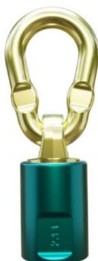
The THEIPA Point-F internal thread attachment swivel is a ball-bearing lifting attachment point for industrial load handling. It is used where a swivel connection with internal thread is required, helping maintain correct load alignment while reducing the risk of link kinking through its crimped link design.
