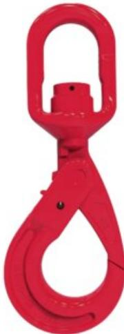
The POWERTEX Self-Locking Hook with a ball-bearing swivel is part of the Powertex G10 Lifting Sling Chain Components range. The self-locking hook closes and locks itself when lifted, making it a safe lifting hook. The hook can be opened by pressing the pawl on the back of the hook. The latch can not be removed. The eye has a ball-bearing swivel and can be rotated both loaded and unloaded.
