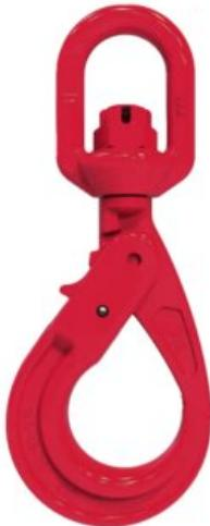
The POWERTEX Self-Locking Hook with slide bearing swivel is part of the Powertex G10 Lifting Sling Chain Components range. The self-locking hook closes and locks itself when lifted, making it a safe lifting hook. The hook can be opened by pressing the pawl on the back of the hook. The latch can not be removed. The eye has a slide-bearing swivel and can be rotated when the hook is unloaded, enabling positioning before lifting.
