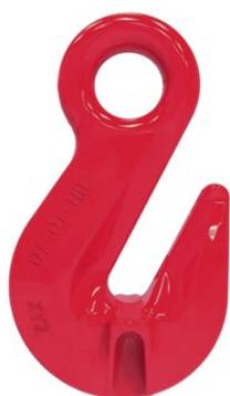
The POWERTEX Grab Hook with eye is part of the Powertex G10 Lifting Sling Chain Components range. The Grab Hook is used for shortening lifting chains, and adding them to an assembly makes the lifting chain assembly much more versatile. It enables full WLL because the support wings prevent the lifting chain from deforming.
