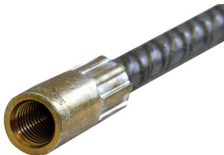
Reinforcement couplings can be used to transfer forces safely between adjacent concrete elements. The reinforcement coupling consists of two elements: threaded inserts (female part) and external threaded pin. Threaded inserts are a composition of threaded inserts clamped on reinforcing steel (for example: Ø12 – M16 for M16).
