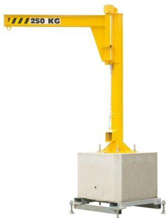
The headroom is the main asset of the PFI MOB. Appropriate for an indoor or outdoor use, its I beam profile allows to consider installation of a hoist with electric or manual steering. This jib crane is mounted on a movable concrete block provided. Displacement can be done by traveling crane (transport ring) or by forklift.
