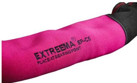
According to EN-1492 regulations for the safe use of round slings, the sling should always be protected at the attachment point (shackle, pin, axle, etc.) as well as at the hoist (crane hook).
