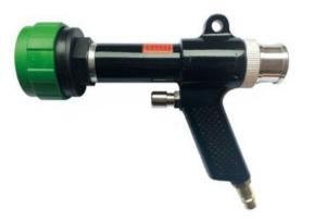
Airgun to dunnage bags allows the user to supply air to the AIRGOBAG, via an Air line. This gun uses a venturi effect to make sure the users does not over fill the AIRGOBAG. Ensuring a safe operation of both products.
