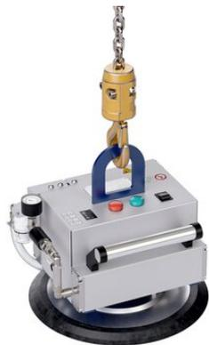
The AERO-CUBE vacuum lifter is a portable lifting device, that is battery-powered. With its compact dimensions and own weight of 20 kilos, it can easily be carried around in your work area without any additional aids. It is provided with two integrated lifting eyes which makes it possible to lift both horizontally as well as vertically. Only thing you need is a lifting device like a crane, pallet truck with a forklift jib, forklift beam or the like.
