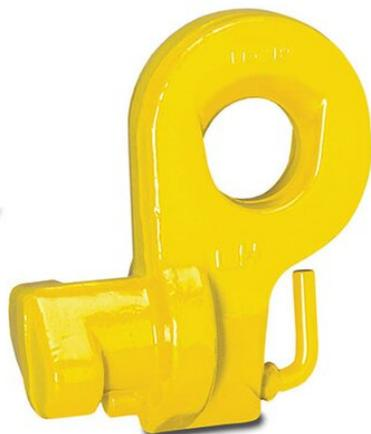
Container lifting lug set for lifting standard containers. They are to be mounted horizontally to the side of the container at either the top or the bottom fixing holes.
