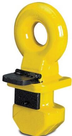
Container lifting lug set for lifting of standard containers in the corner fittings on top. Only for vertical lifting slings. A set contains 4 lugs and are to be used together with a lifting beam. The lugs suits standard ISO corner boxes.
