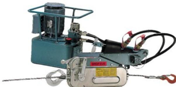
Hydraulic Tirfor machines are portable motorised hoists used with maxiflex wire rope. They can be used to lift, pull and position loads over great distances depending on the wire rope length. They are suitable for use in numerous configurations and are the ideal solution for use in professional applications; they are operated by an hydraulic cylinder powered by either an electrical power pack or a petrol motor power pack
