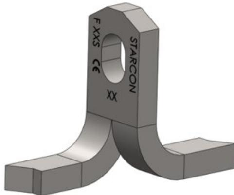
Starcon STA-F, also known as the flat-foot anchor, is ideal for slab, floor and deck elements. As the feet are parallel to the surface, this provides a strong anchorage in thin elements. At the top of the STA anchor, a hole is located for attaching a ring coupling. Reinforcement can be easily and clearly placed on the top of the feet. Designed for large, thin prefabricated elements that are lifted perpendicular to their main surface, this anchor is a robust alternative to the STA-P plate anchor.
