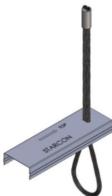
The Starcon wire box consists of a high-strength steel wire rope and a steel box and is used in concrete elements when these are to be mounted next to each other. It is installed in concrete elements before pouring.
