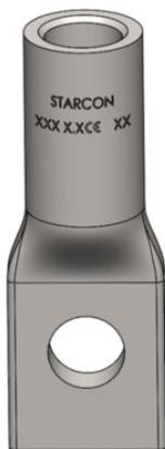
The Starcon cross-hole transport anchor is designed with an internal thread for transporting and fastening concrete elements. The transport anchor is always used in conjunction with additional reinforcement, which is bent and installed in the lower cross hole.
