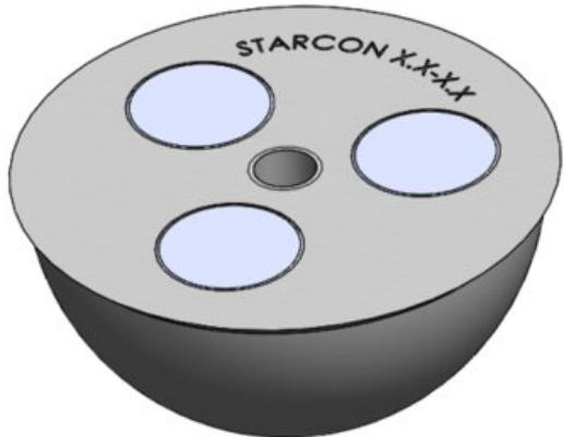
Starcon steel former are available with and without magnetic accessories to streamline the disassembly process. They are designed in a hemispherical design, where the spherical anchor can be easily placed in the former and then in the concrete element before pouring.
